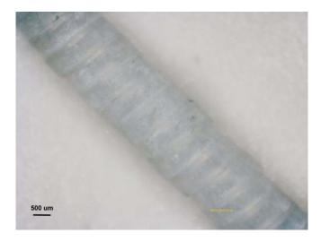
**Fig. S6.** Photograph of the helical PDMS substrate with ZnO nano-aggregates grown on it *via* a hydrothermal synthesis.
